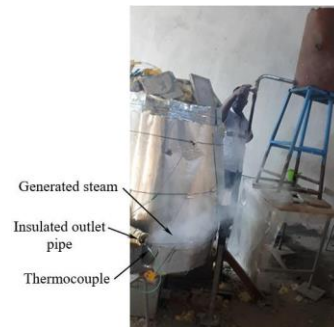
Figure 11: TES discharging with load using water. A thermocouple was installed at the outlet of the heat-extracting pipe to measure the temperature of the outgoing generated steam leaving the system (Figure 11). The discharging process continued until the steam temperature dropped below a certain threshold, showing that the stored thermal energy was no longer able to produce steam.
