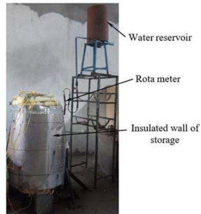
Figure 10: The water reservoir used during the discharging phase of the thermal energy storage (TES) system. This reservoir, positioned above the TES, supplied the water that was heated by the stored thermal energy.
