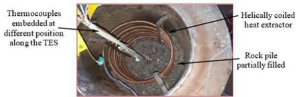
Figure 7: Internal part of the TES before fully filling the rock piles
