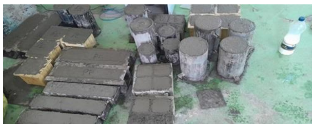
Figure 2. Concrete test samples for mechanical property determination.
