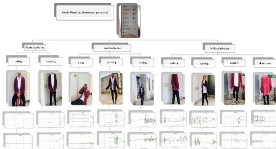
Fig. 2. Logical flow of the data collection process showcasing a volunteer participant with corresponding accelerometer and gyroscope data
