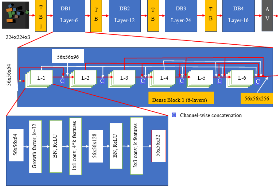
Fig. 9. A deep DenseNet-121 with four dense blocks
